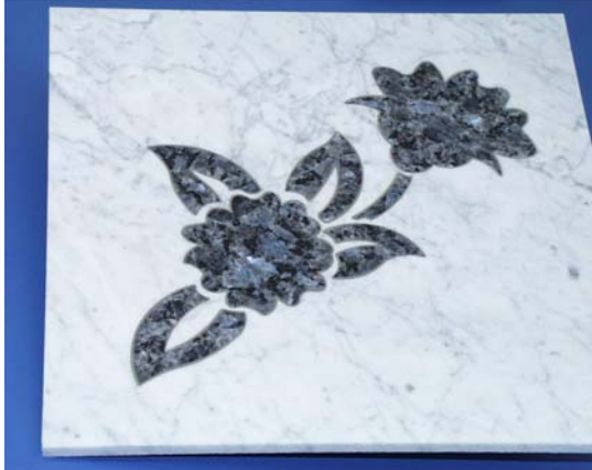
Fig. 16 The Labrador flower was inserted in a Marble tile at KMT Waterjet
