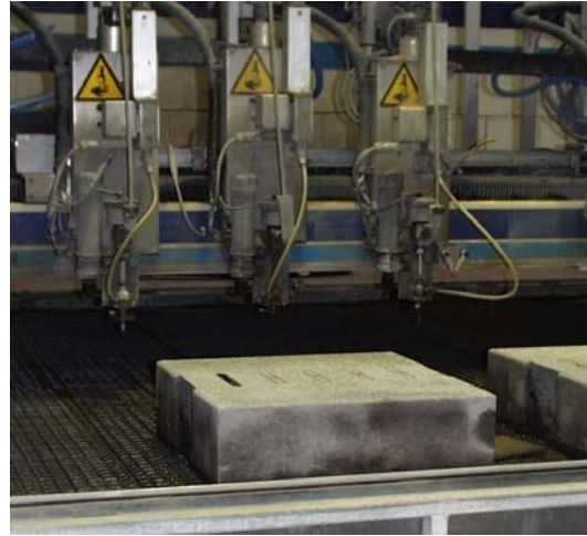
Fig. 14 180mm thick concrete plates cut at KMT Waterjet, Bad Nauheim
